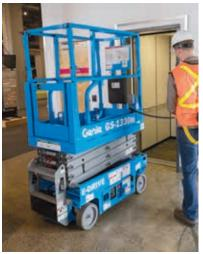
This lightweight scissor lift is able to access jobsites previously off limits to heavier slab scissors and vertical mast lifts in the industry due to passenger elevator capacity limitations
