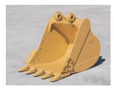
**Heavy-Duty (HD) Buckets.** Heavy-Duty (HD) buckets for digging in moderate to hard abrasive materials feature large Ground Engaging Tools (GET), thick cutting edges and thick bottom and side wear plates to improve performance in demanding conditions.
