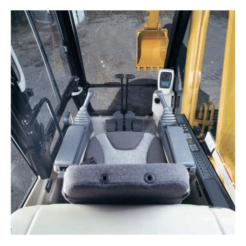
**Operator Station.** The 320C operator work station is quiet with ergonomic control placement and convenient adjustments, low lever and pedal effort, ergonomic seat design and highly efficient ventilation.
