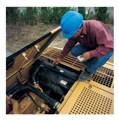
**Diagnostics and Monitoring.** The 320C is equipped with S•O•S<sup>SM</sup> sampling ports and hydraulic test ports for the hydraulic system, engine oil and for coolant. A test connection for the Cat Electronic Technician (Cat ET) is located behind the cab.
